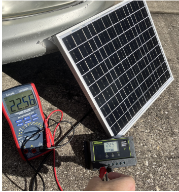
Figure 88: Solar Panel Voltage Testing
