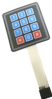
Figure 18: 12 Key Membrane Switch Keypad
