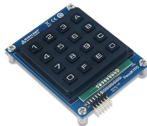
Figure 20: Digilent PmodKYPD - 16-button Keypad
